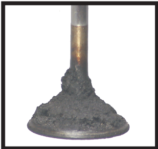
Dirty Intake Valve
